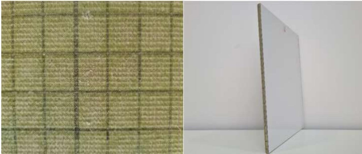
Detail of the core of the multi-layer panel (left), overview of the sandwich panel (right).
