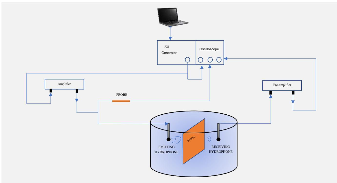
Schematic of the layout and connection between equipment involved in the test.
