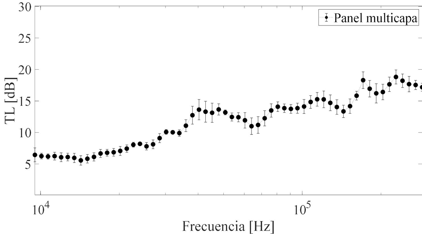
Measured transmission losses with the multilayer panel
