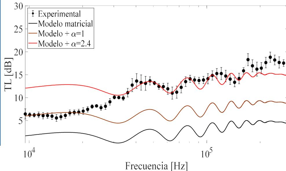
The measurements give higher values than the theoretical values (black line) which may be due to additional absorption in the panel either because it is not a strictly homogeneous solid panel as modelled or even because of the presence of (highly reflective) air micro-cavities inside the panel.
