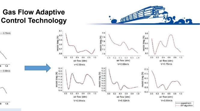
Utilizing this test data as a sample, the resistance of the model was calculated by using a 4-layer BP neural network algorithm.
