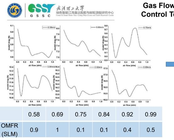
Microbubble drag reduction effectively reduces the sailing resistance.
